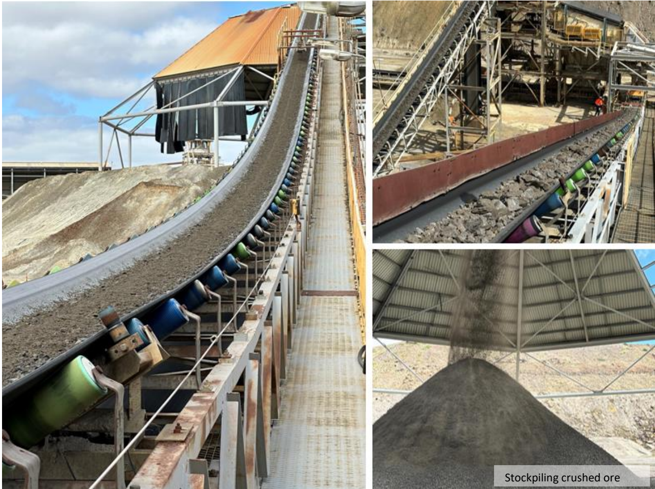
Figure 2 Stockpiling crushed ore in preparation for copper production
